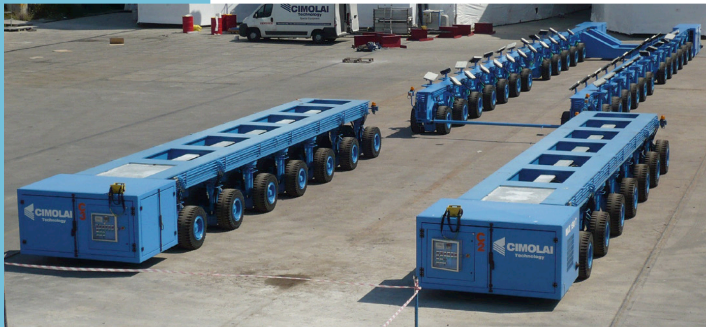
Capacity: 750 t (350 t + 2x200 t) - ITALY Electronic steering system on all wheels
